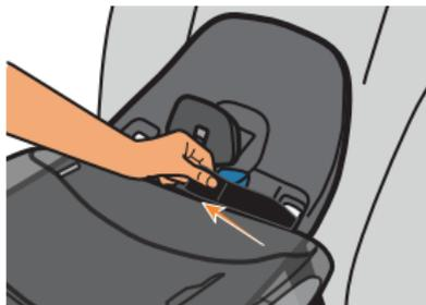
7. Press down on the sides of the SafeLock Belt Tensioner until an audible **CLICK** is heard. If Belt Tensioner does not lock, try loosening the LATCH/UAS Strap slightly, then try to close again.
